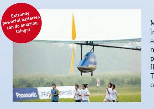
More than 100 years after the Wright Brothers succeeded in the world's first manned flight, Panasonic Batteries and the Tokyo Institute of Technology (TIT) have marked a milestone in aeronautic history. In July 2006, an airplane powered by 160 Panasonic AA Digital Xtreme Power batteries flew a distance of 391,4 metres at an altitude of 5,2 metres. The one-seat airplane, weighing 107 kg with a wingspan of 31 metres, was in the air for 59 seconds.
